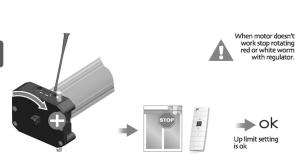
Using special regulator to adjust "+" direction, and rotating white worm when need to increase the up distance worm and press the stop button
